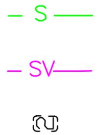
— S — 4/0 TPX SECONDARY CABLE BY PG&E IN APPLICANT INSTALLED 3" CONDUIT.
